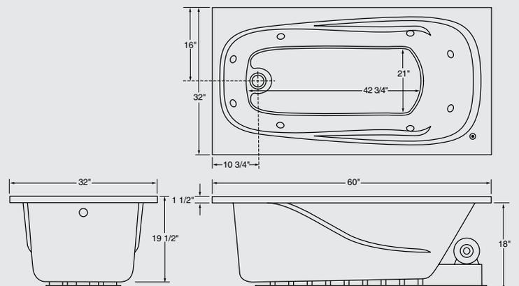
NOTE: All dimensions and specifications are nominal and may vary  $\pm 1/4"$ . Use actual products for accuracy in critical situations. All whirlpools require a single 115V/20 amp GFCI circuit.
